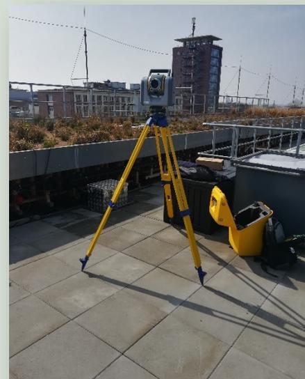
Figure 3: Trimble SX10 scanning total station on the research canopy
