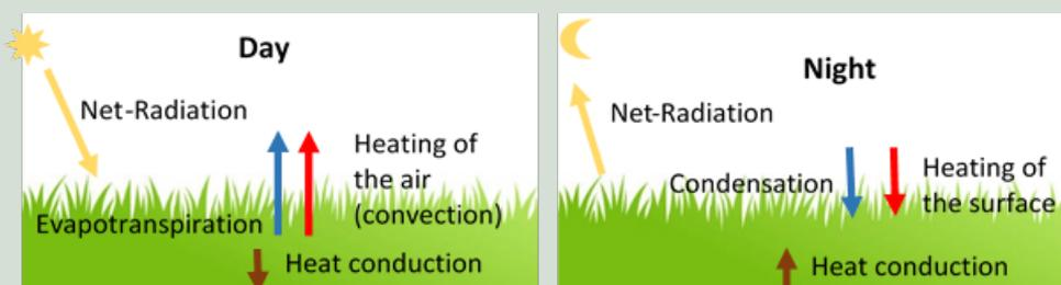
Figure 1: Schematic representation of the surface energy balance
